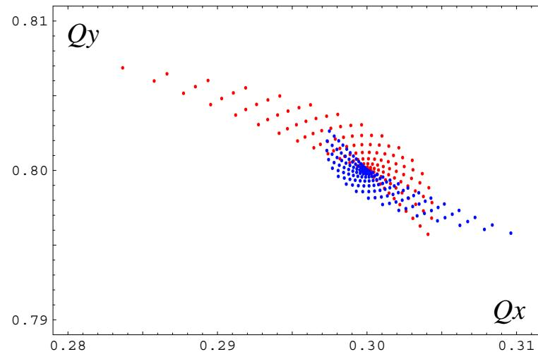
Figure 10: Comparison of tune-shift plots using body (red) and local (blue) compensation of the dodecapole component in the SNS ring quadrupoles.
