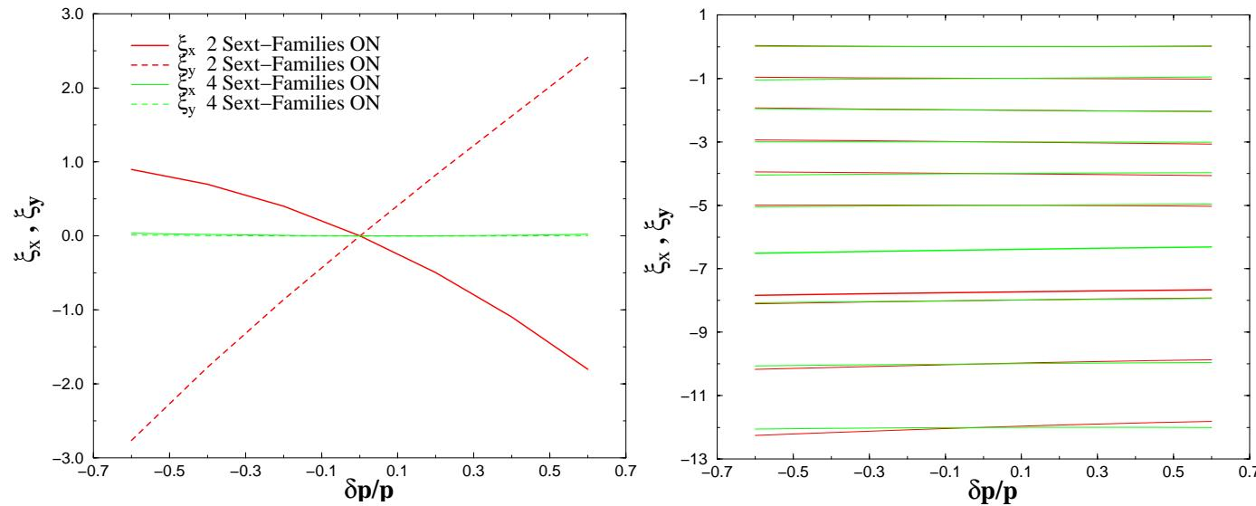
**Figure 4:** Plot of the chromaticities  $\xi_{x,y,T}$  as a function of momentum spread, when four families of sextupoles are used. The natural chromaticities are also plotted (distinct red and green lines in the middle of the plot). This plot reflects the successful minimization of the first and second order chromatic terms, accomplished by the four sextupoles families' scheme.
