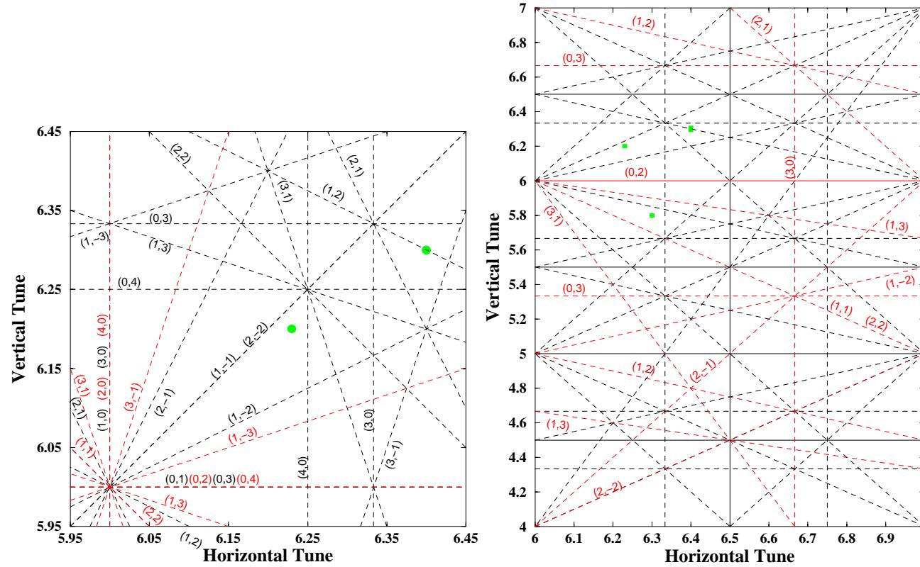
Figure 1: Tune spaces for a lattice with super-period four. The red lines are the structural resonances and the black are the non-structural (up to 4th order).
