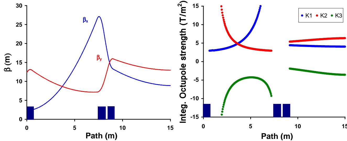
Figure 8: Top: the  $\beta$  functions in the first half of the SNS straight section. x Bottom: integrated strengths of three families of octupoles versus location of the third family.
