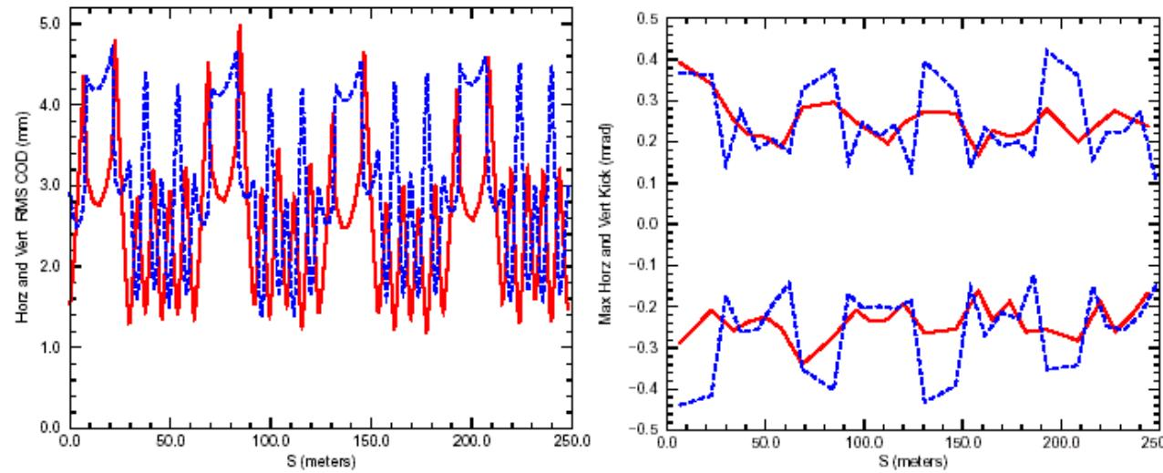
Figure 2: Horizontal and vertical closed orbit rms displacement for 101 error distributions in the SNS accumulator ring and maximum kicks required for correction (courtesy of C.J. Gardner)
