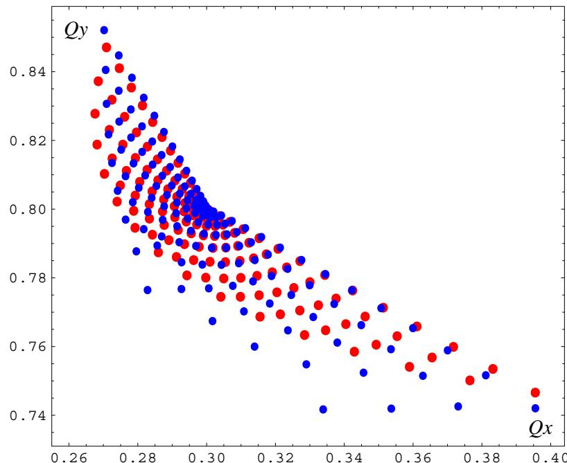
Figure 9: Tune footprints of a ring lattice with a dodecapole error in the quadrupoles of  $b_5 = 60$  units; results are from tracking data (blue) or the analytic estimate (red).
