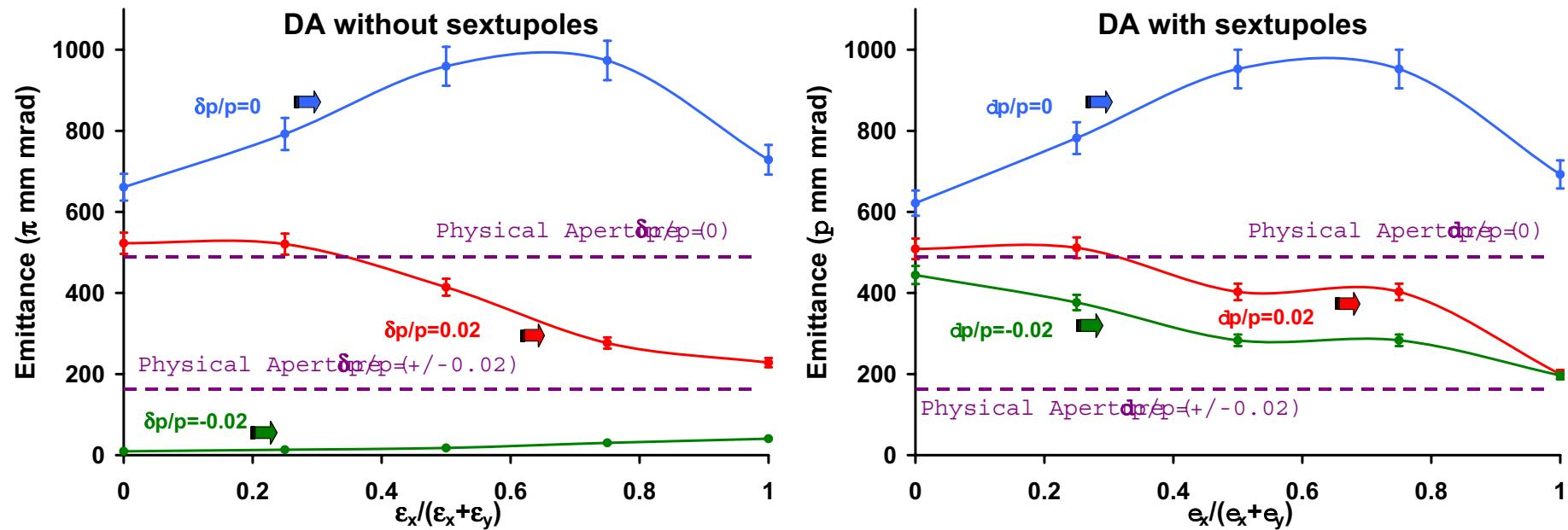
Figure 11: Dynamic aperture for the working point (6.3,5.8), without (left) and with (right) sextupoles.
