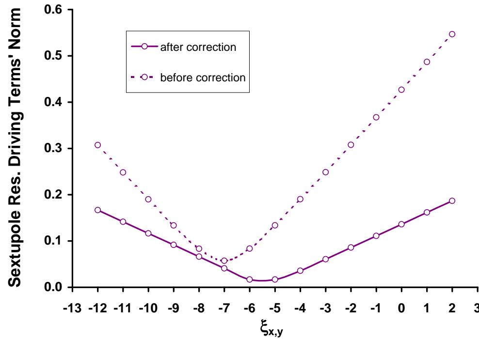
Figure 7: Norm of sextupole resonance driving terms before correction (dashed line) and after correction (solid line) with dedicated sextupole correctors. The resonance norms are reduced after the correction by as much as a factor of four.
