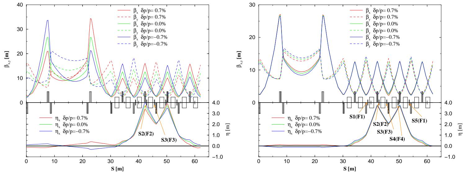
Figure 3: Lattice functions of a ring lattice using two (left) and four (right) families of sextupoles.
