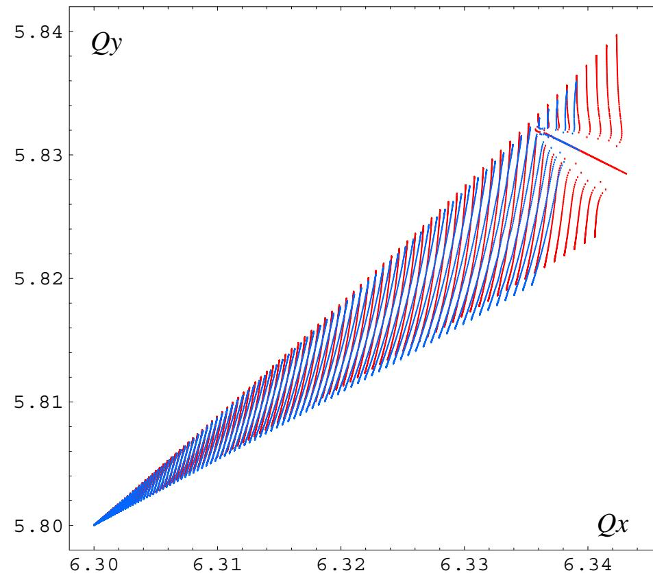
Figure 5: Tune footprints of the SNS ring, based on realistic (blue) and hard-edge (red) quadrupole fringe fields.
