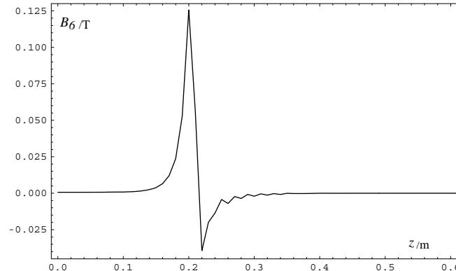
Figure 6: Dodecapole component in a 21 cm quadrupole with un-shaped ends. The reference radius is 10 cm, and the origin,  $z = 0$ , is at the magnet's center.
