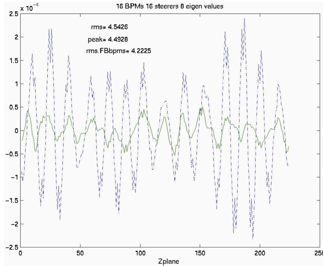
Vertical orbit correction with 16BPMs and steerers
