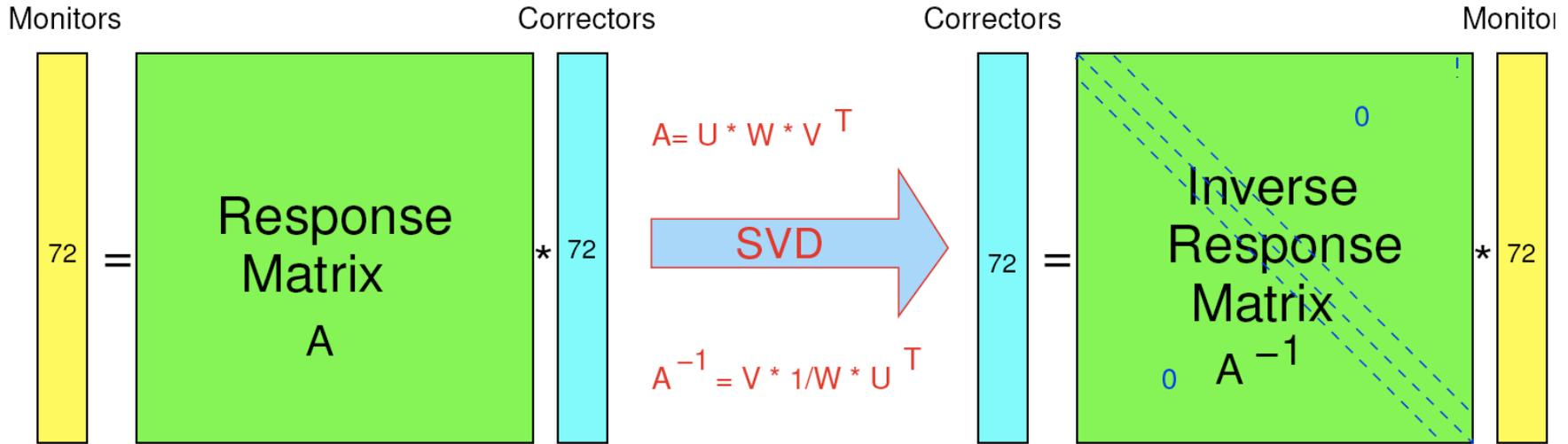
=> Minimization of the RMS orbit (=0 in case of "Matrix Inversion" using all Eigenvalues)
