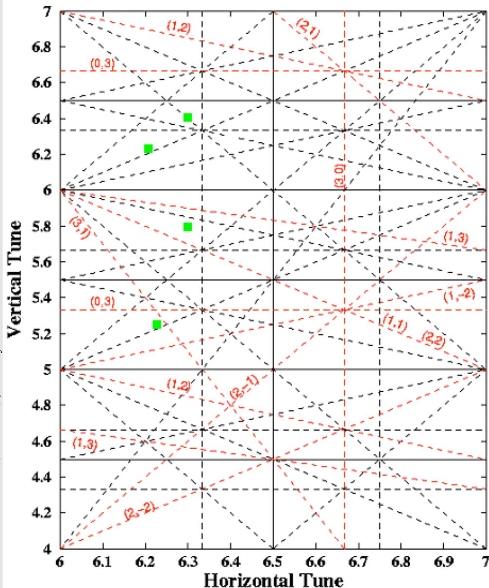
Tunability: 1 unit in horizontal, 3 units in vertical (2 units due to bump/chicane perturbation)
